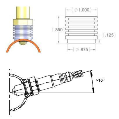
FIGURE 2. Sensor Bung and Sensor Mounting
