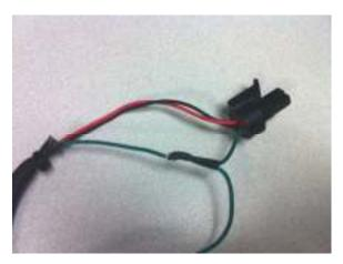
Figure 7. Cut & Spliced wires
