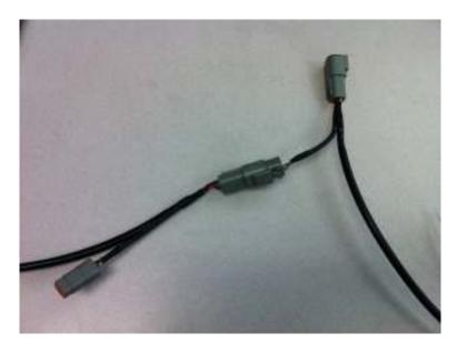
FIGURE 11. AEMNet cable connection
