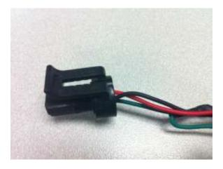
Figure 6. EBP sensor connector
