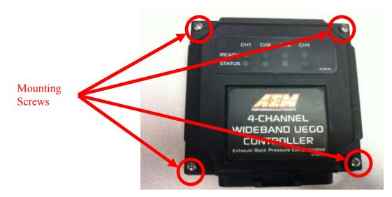
FIGURE 3. Mounting holes
